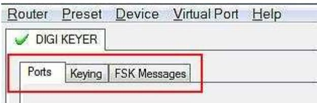
Router must be used to configure DIGI KEYER for proper operation. The device configuration tab (in the red rectangle) is used to setup each part of the DIGI KEYER – virtual ports for communicating with the application (Ports), audio levels, PTT and keyboard FSK (Keying), and stored FSK messages (FSK Messages).
