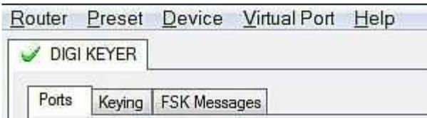
When the USB driver is installed correctly and DIGI KEYER is powered from a radio or external 12V DC supply Router will show a device tab with a **GREEN** check beside the device name (DIGI KEYER).
