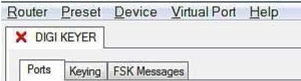
When Router shows a **RED** "X" instead of a green ✓, it means the device is disconnected and Router does not see the USB part of DIGI KEYER.
