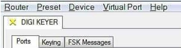
When Router shows a **YELLOW** "X" instead of a green ✓, it means the USB driver is correctly installed but DIGI KEYER is not receiving power from the radio or external supply.
